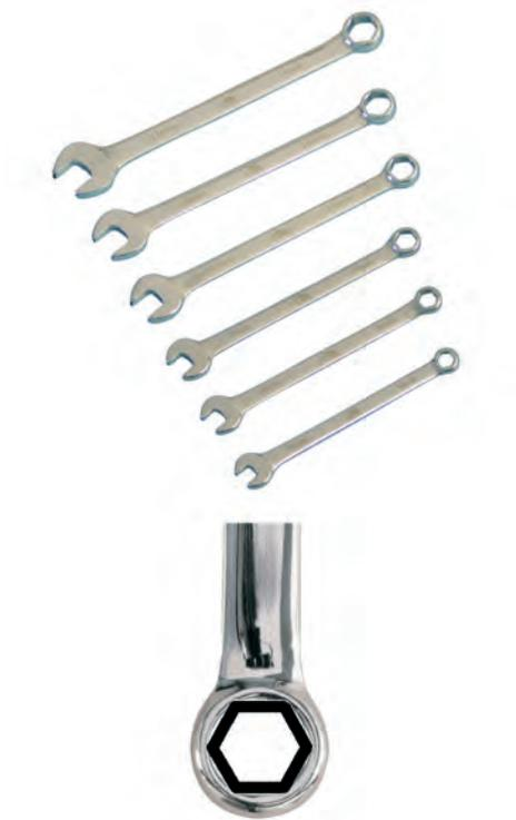
ATE bleeder wrenches can be used to open and close all common bleed valves easily and without damage thanks to the internal hexagon of the ring end that is angled by 10°.
