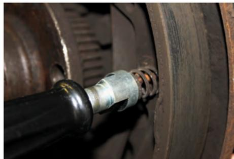
The ATE spring mounting tool is used for the safe and problem-free removal and mounting of the retaining plates of brake-shoe retaining springs. Two different size seating bells safely accommodate large and small spring plates of the brake-shoe retaining springs.
